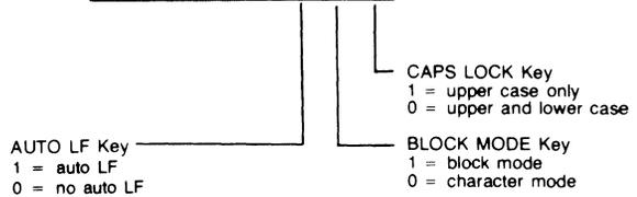
**BYTE 1 KEYBOARD INTERFACE SWITCHES (A-D)**
