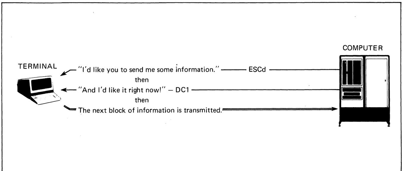
Figure 5-3. Block Transfer Enabled By The Computer
