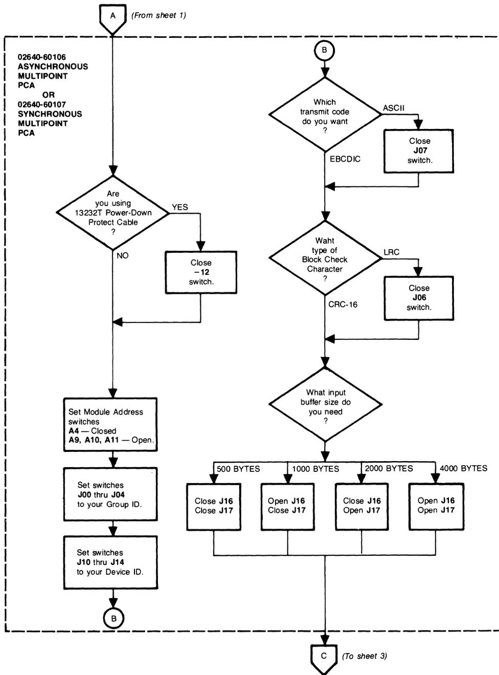
Figure 5-17. Multipoint Data Communications Configuration (Sheet 2 of 4)
