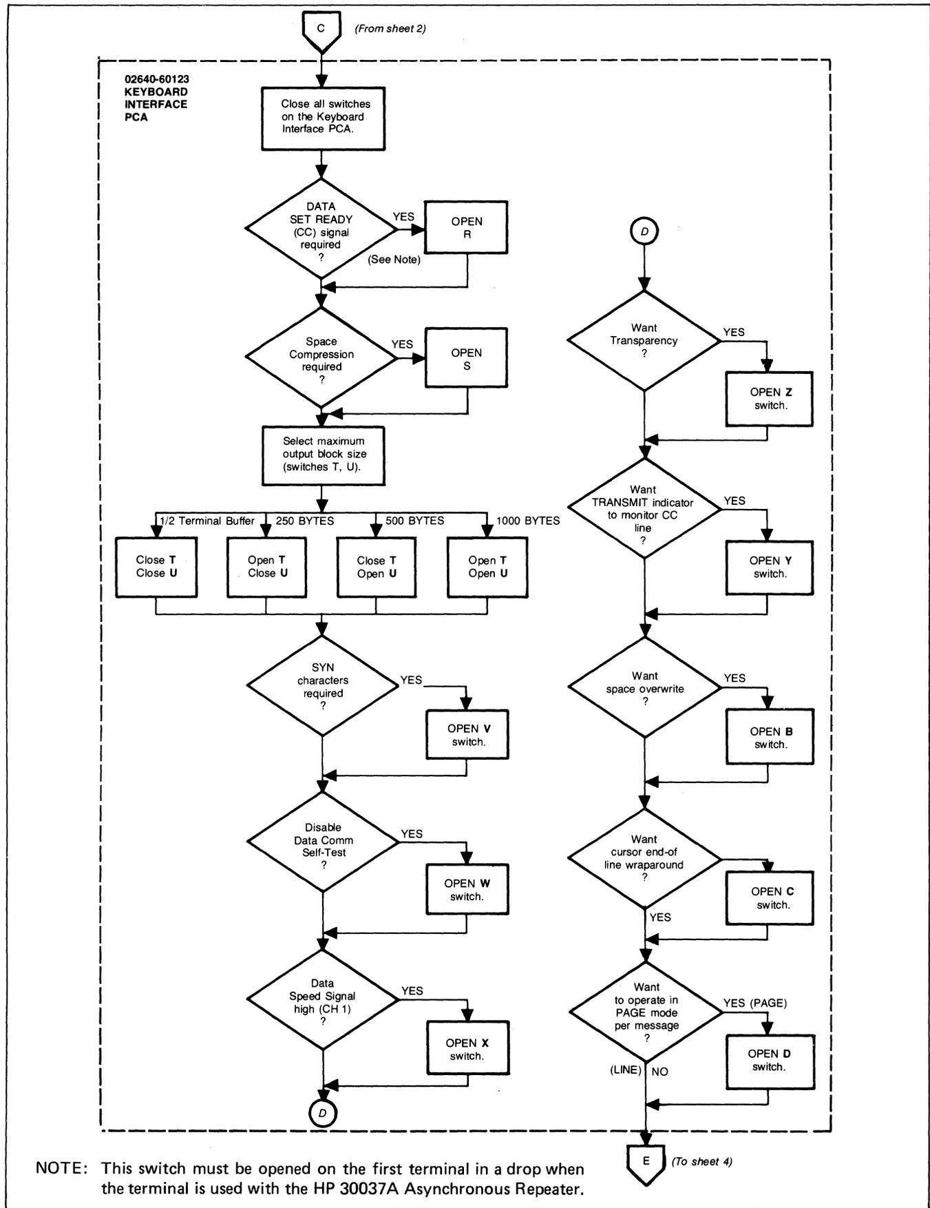
Figure 5-17. Multipoint Data Communications Configuration (Sheet 3 of 4)
