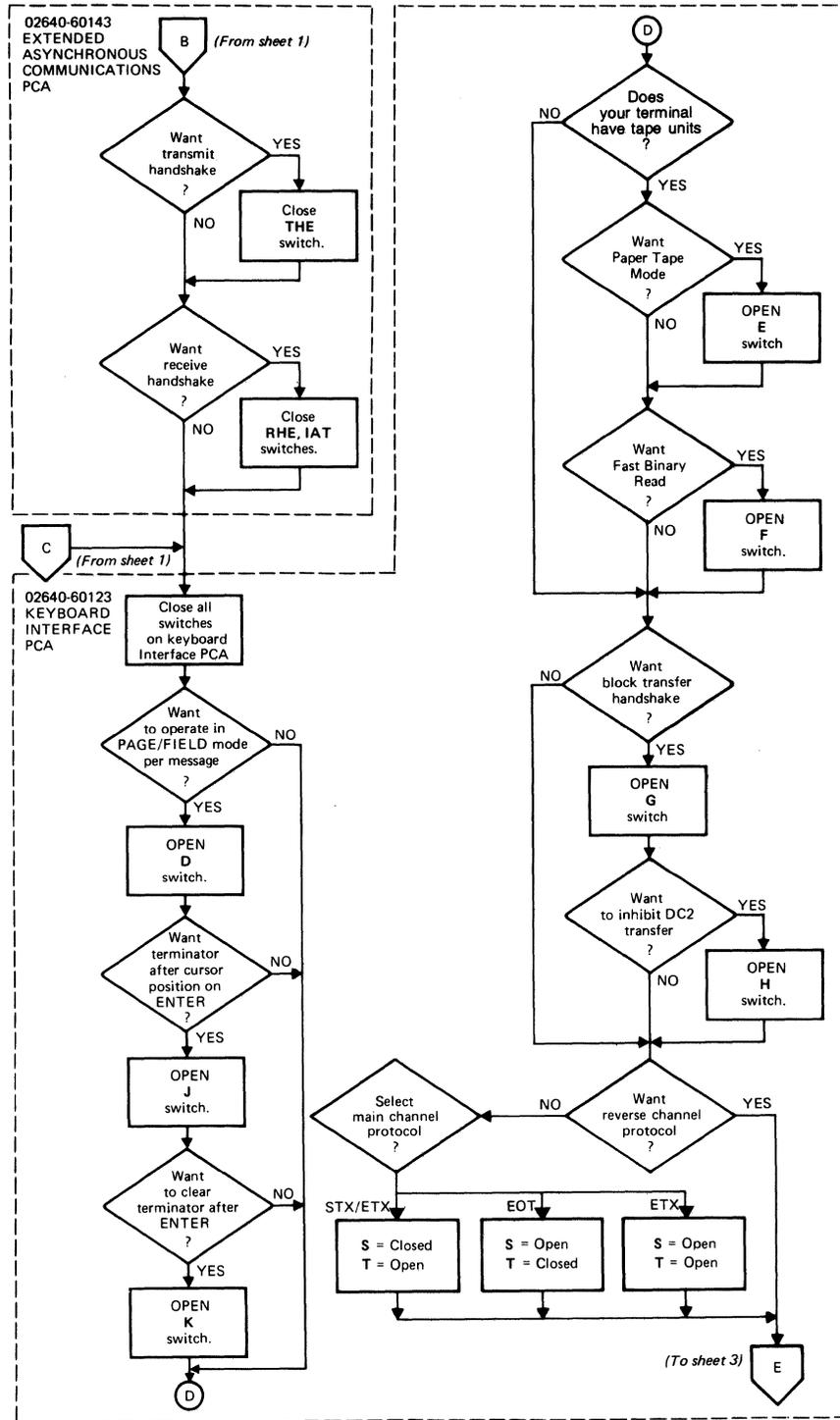
Figure 5-10. Point-to-Point Data Communications Configuration Flowchart (Sheet 2 of 4)
