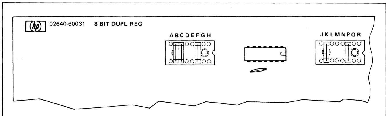
Figure 7-11. Terminal Duplex Register PCA Jumper Configuration
