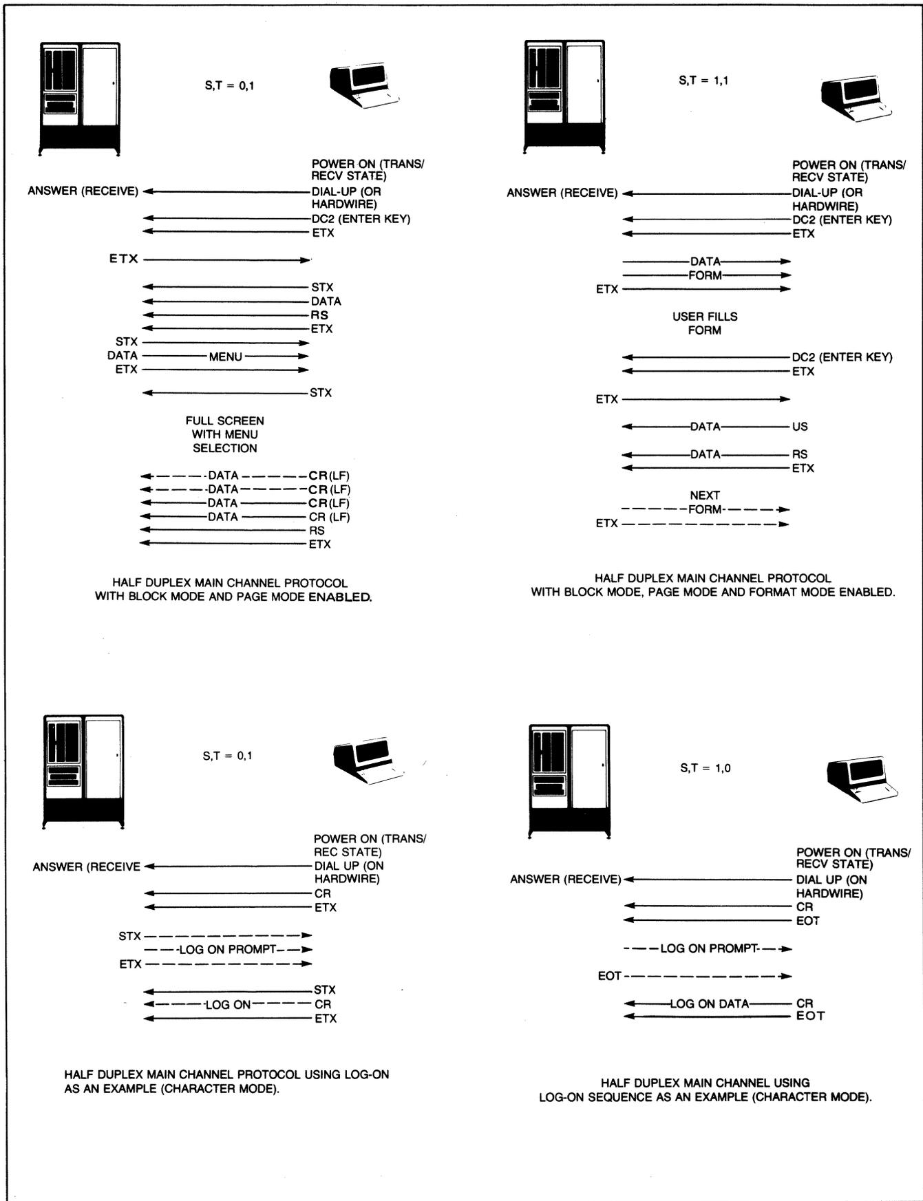
Figure 5-7. Sample Data Transfers Using Main Channel Protocol
