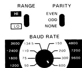
Figure 5-13. Block Keyboard Data Communication Switches
