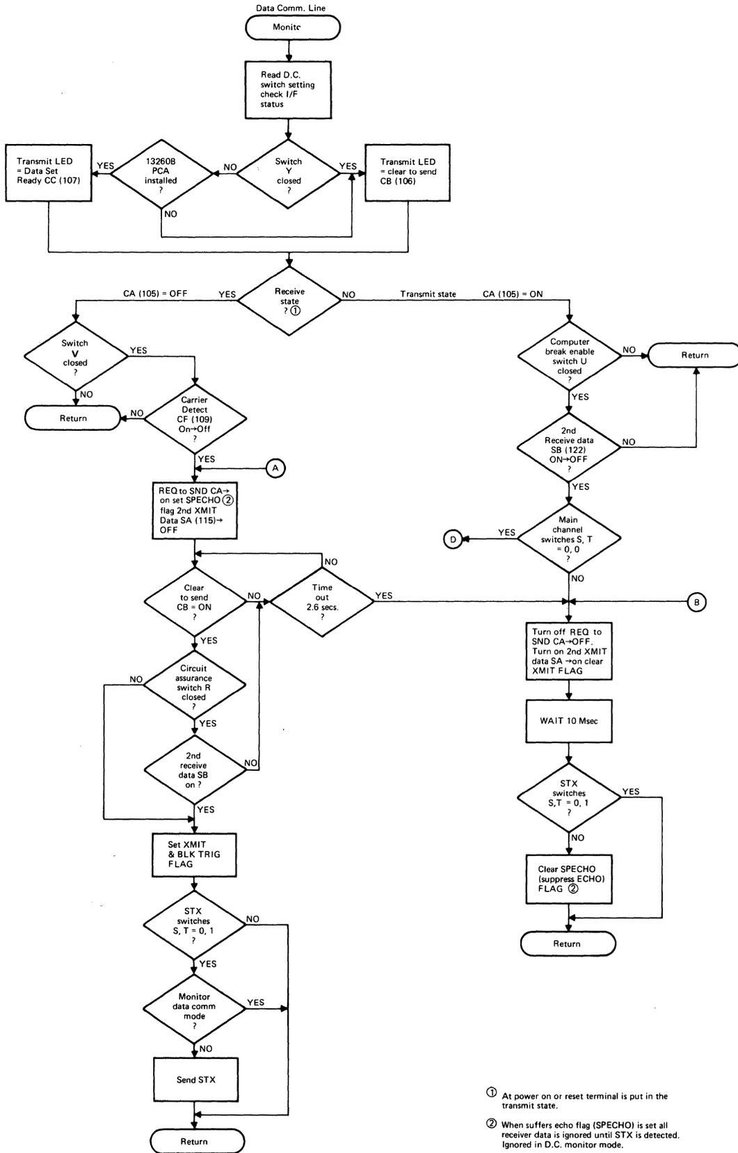
Figure C-1. Point-to-Point Communication Flowcharts (Sheet 1 of 3)
