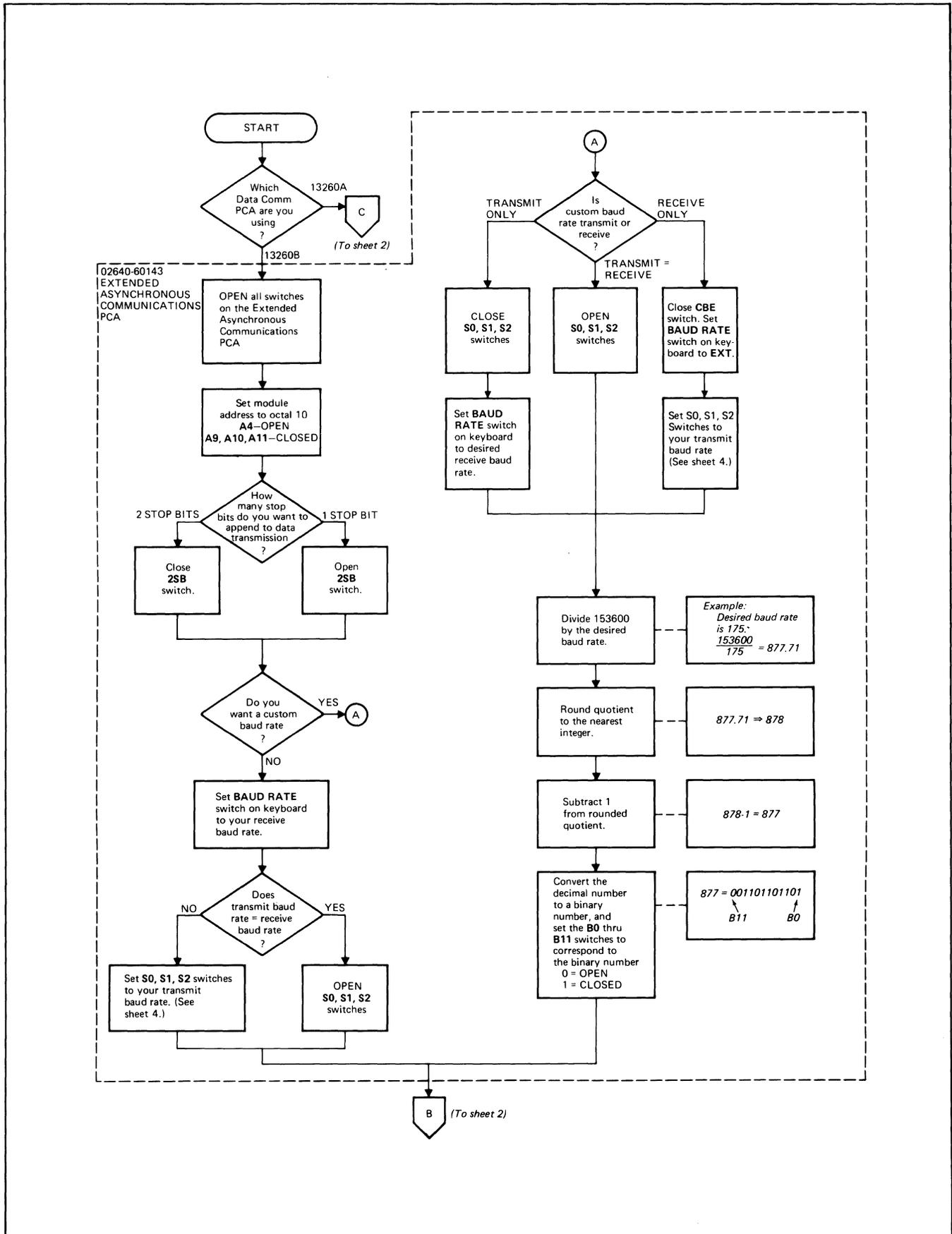
Figure 5-10. Point-to-Point Data Communications Configuration Flowchart (Sheet 1 of 4)
