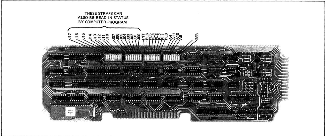
Figure 7-17. Asynchronous Multipoint Communications PCA Strapping Options
