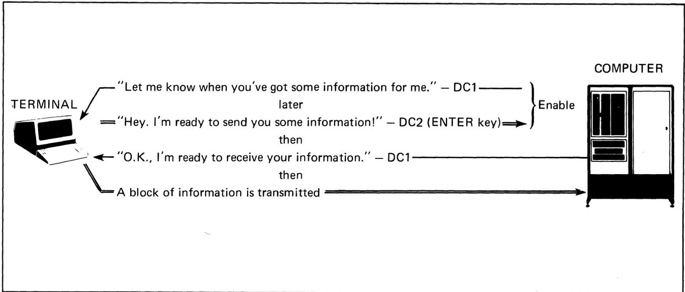
Figure 5-2. Block Transfer Enabled By The ENTER Key
