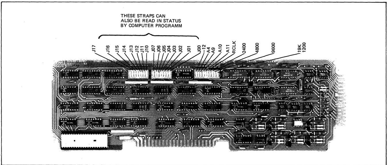
Figure 7-18. Synchronous Multipoint Communications PCA Strapping Options
