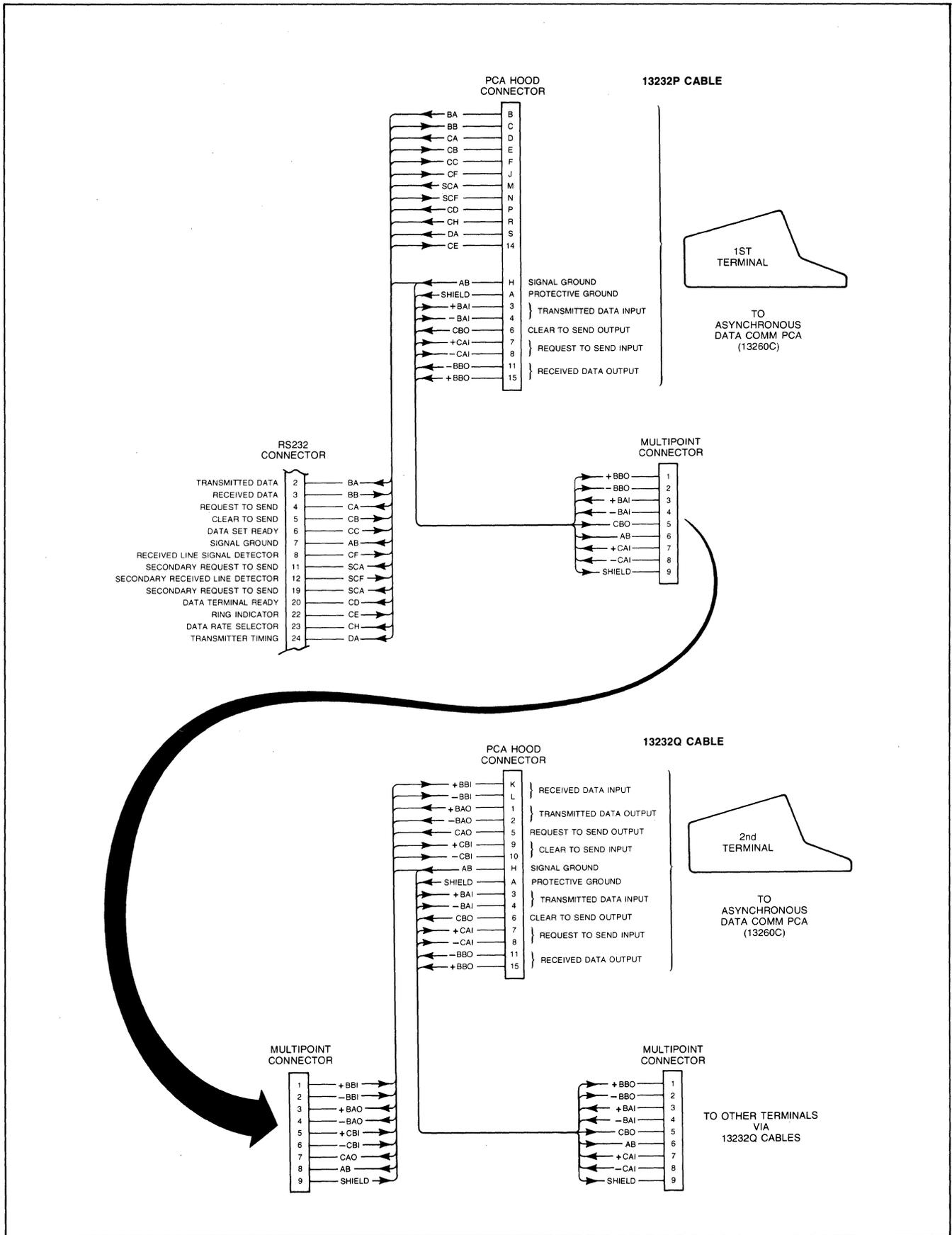
Figure 7-22. Asynchronous Multipoint Cabling
