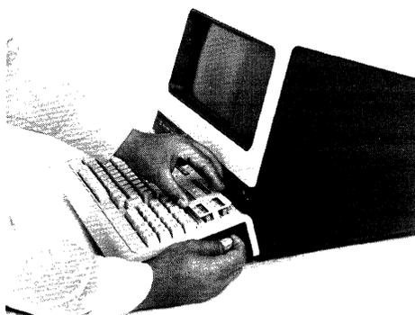
A. REMOVING A KEYBOARD OVERLAY
