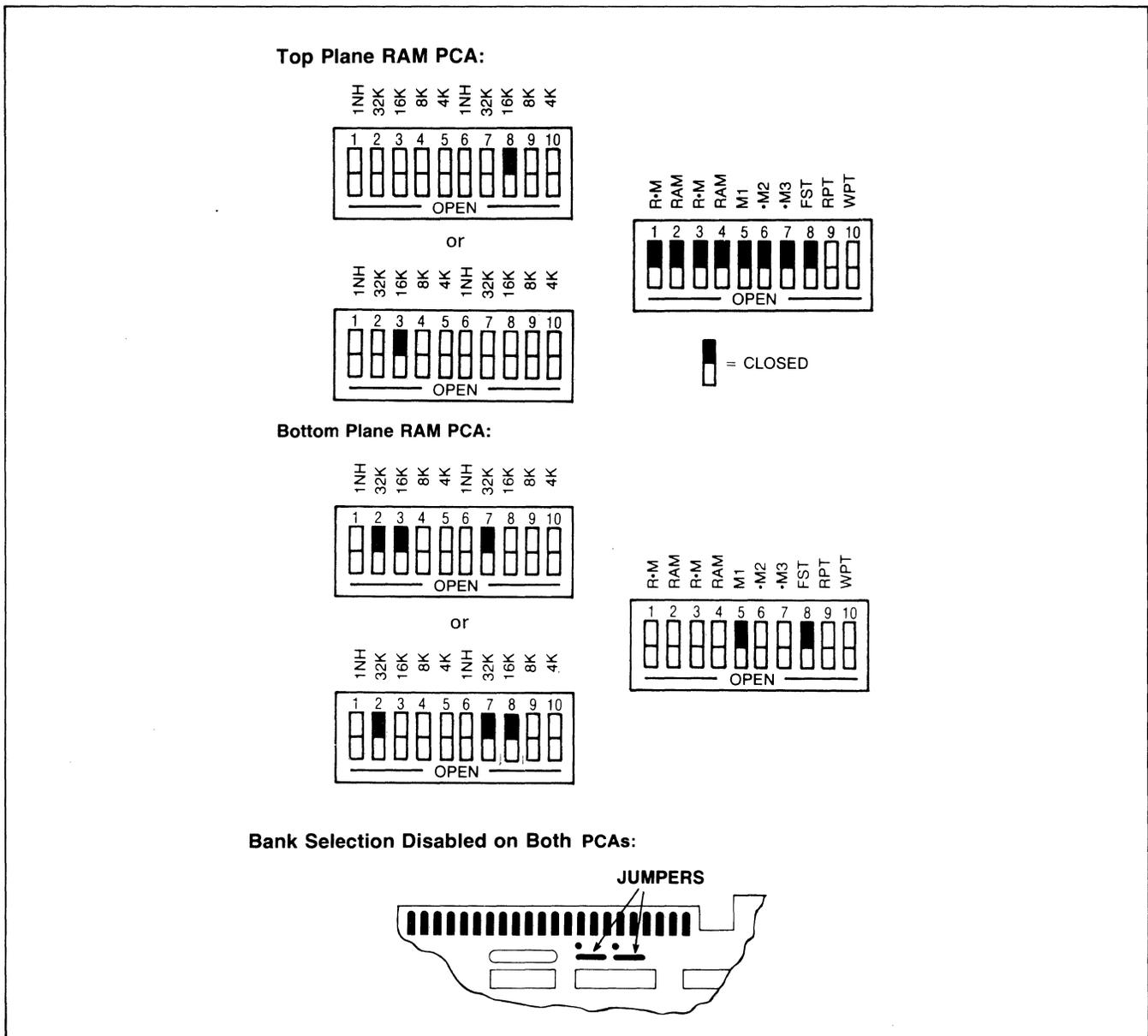
Figure 7-8. 32K RAM PCA Jumper Settings
