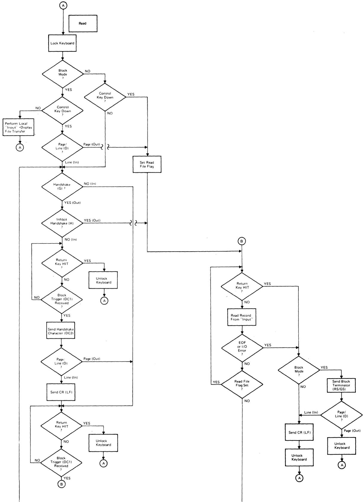
Figure C-2. Keyboard Communication Switches Flowcharts (Sheet 3 of 4)
