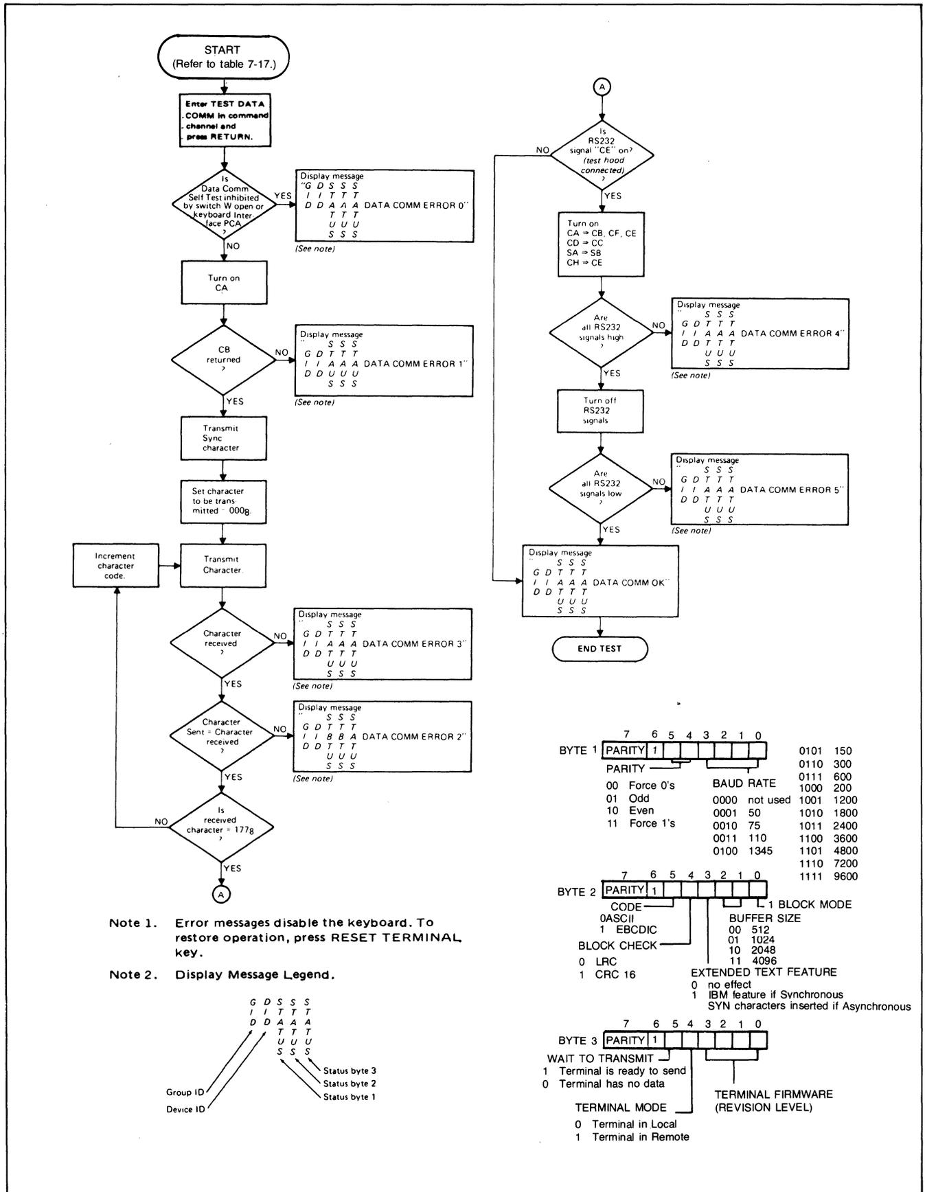
Figure 7-32. Multipoint Data Comm Self-Test Flowchart
