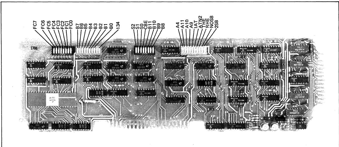
Figure 7-16. Extended Asynchronous Communications PCA Strapping Options
