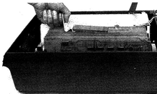
Figure 7-7. Top Plane Assembly Removal
