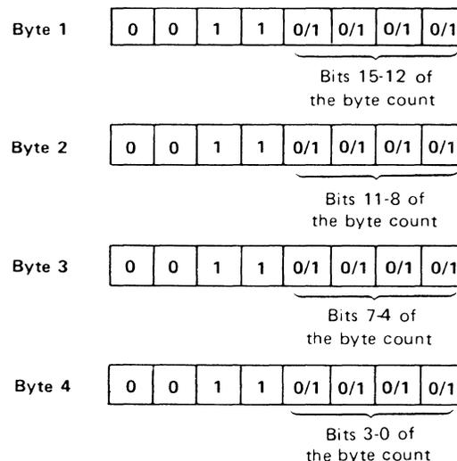
To transfer binary data, the read control byte in the escape sequence must specify a byte count (2R or 3R), and the PARITY switch on the terminal must be set to NONE. If a non-recoverable error occurs, the terminal will send an RS/GS as if a file mark were detected. The type of error can be determined by inspecting the device status.
