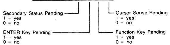
**BYTE 2 KEYBOARD INTERFACE SWITCHES (E-H)**
