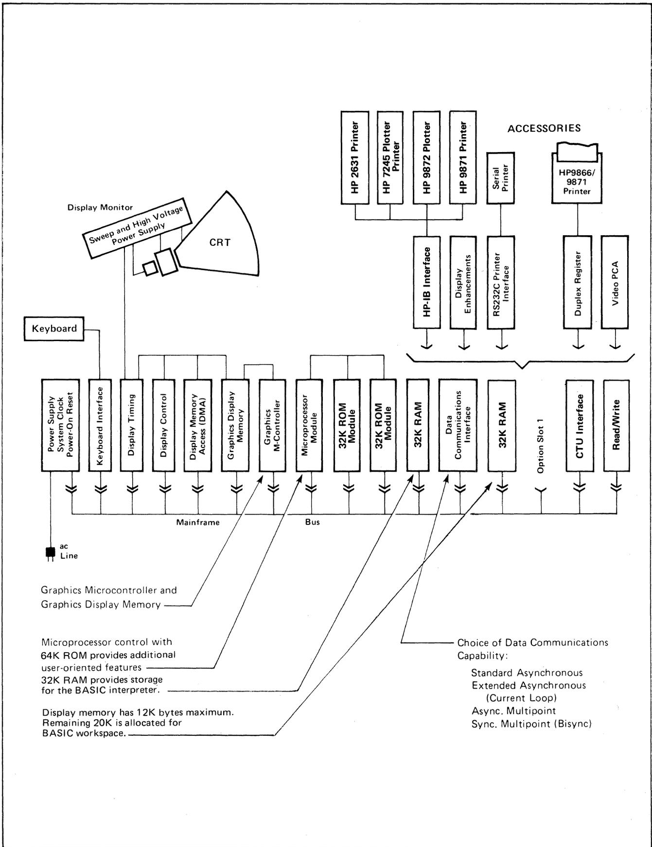
Figure 1-1. Terminal Architecture
